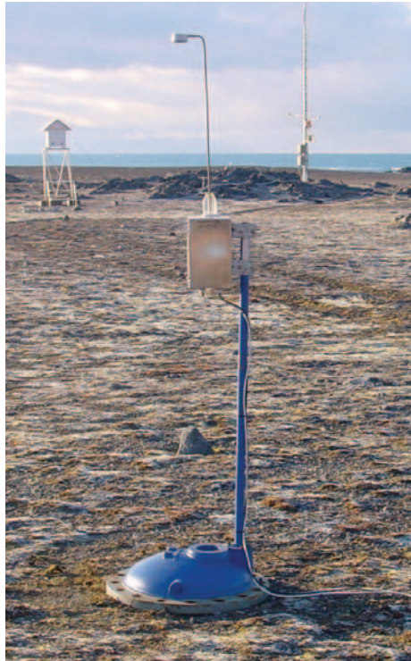
Fig. 5. The radioactive collector for electric field measurement at the Polish Polar Station Hornsund, Spitsbergen.
