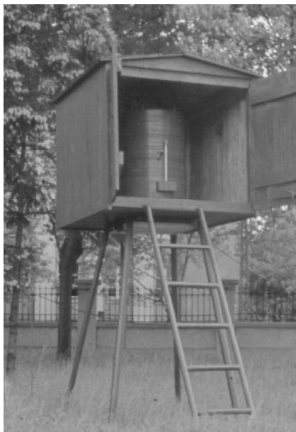
Fig. 1. Housing of the gamma radiation detector made of a steel slab from the wrecked ship.
