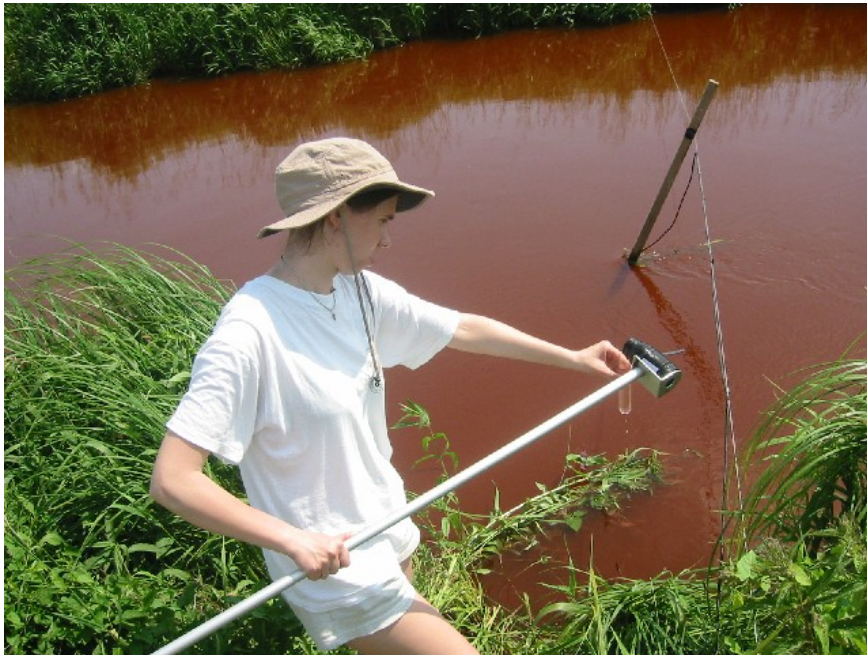
Figure 2.6: Tracer test performed in a natural Narew river in the North-East of Poland in June 2005 (Rowiński et al. , 2007, 2008); after complete mixing along the river width
