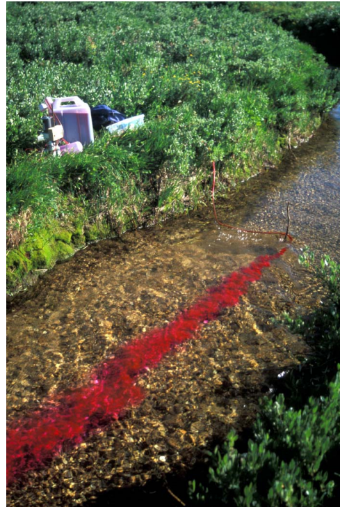
Figure 2.3: Rhodamine dye study of hydrology of stream-lake interactions (Spring Creek lake); source: http://www.aslo.org/ , author: Prof. Wayne Wurtsbaugh
