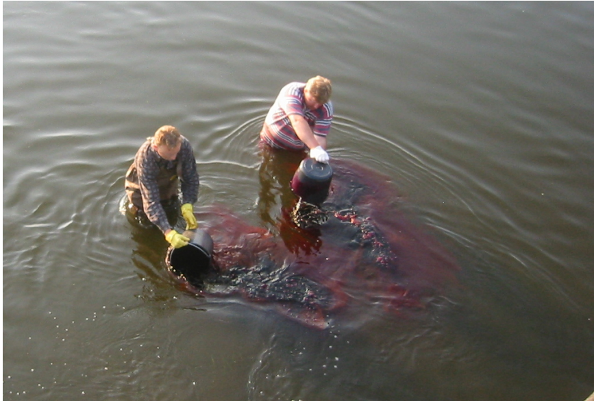
Figure 2.4: Tracer test performed in a natural Narew river in the North-East of Poland in June 2005; dye release
