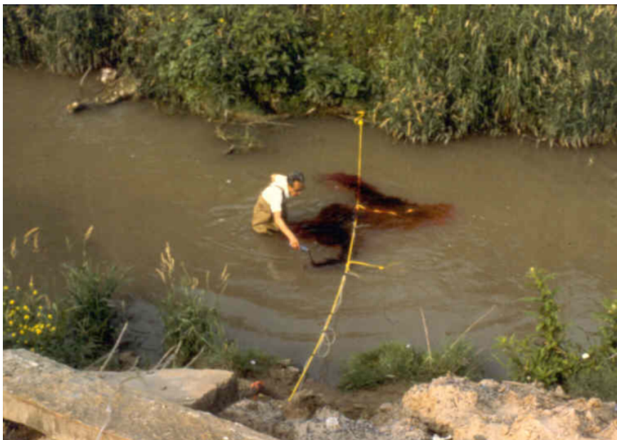
Figure 2.5: Tracer test performed in a small river (river width: B = 5 m, height: H = 1 m); dye release; source: (Holley, 2001)
