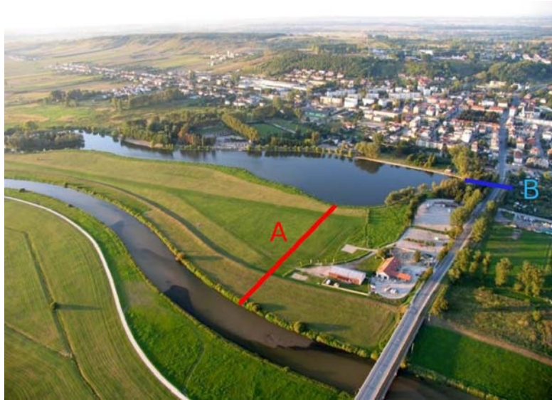
Fig. 2. The reservoir and the Nida River with visible bedforms (photo: Aeroklub Pińczowski). A – proposed channel, B – existing channel.
