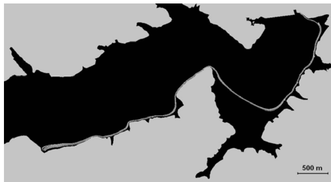
Fig. 3. Tracking of pollutants entering the lake from the tributary 5. The situation after 125 hours from the event of entering the lake by the pollutants.
