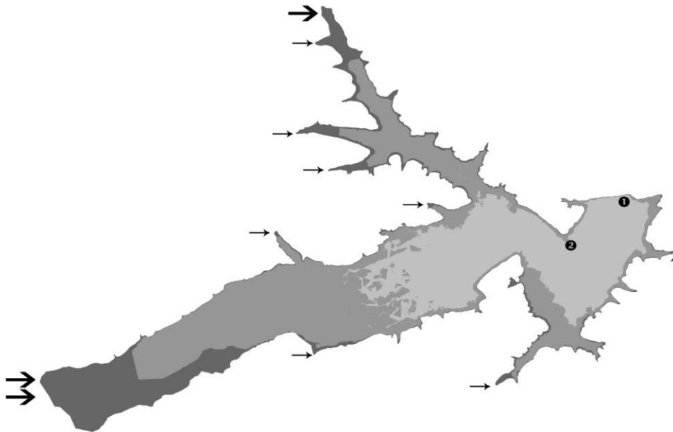
Fig. 1. The shape of the Dobczyce lake at different water levels: minimal (light grey), average (grey), and maximal (dark grey). The ❶ symbol shows the position of dam inlets while the ❷ symbol denotes the location of the water supply inlet. The double bold arrow indicates the main inflow (Raba), the single bold arrow indicates the biggest side inflow (Wolnica), while the thin arrows indicate a few of other inflows (minor creeks).
