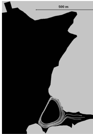
Fig. 5. Tracking of pollutants entering the lake from the tributary 7. The situation after 120 hours from the event of entering the lake by the pollutants. Most of the tracking particles are caught by the clockwise whirl.
