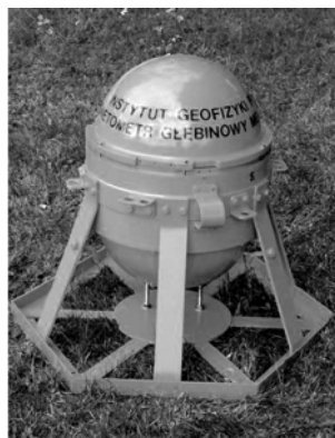
Fig. 1. The bottom magnetometer MG-01/2003 in its capsule.
