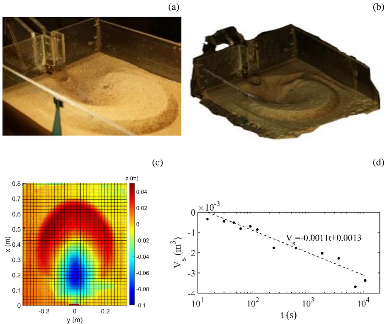
Fig. 1: (a) Photo of the spillway and dissipation basin, (b) obtained 3D model, (c) quantitative results of scour cavity and bar topography, (d) time evolution of the scour for  $Q = 0.85 \text{ Ls}^{-1}$  and  $h = 0.05$  m.
