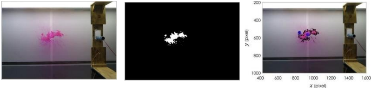
Fig. 1. Identifying the spill by imaging methods. From left to right: raw image, binary image, isolated spill.
