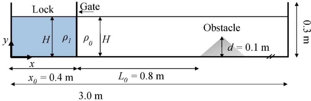
Fig. 1. Schematic representation of the experimental apparatus.
