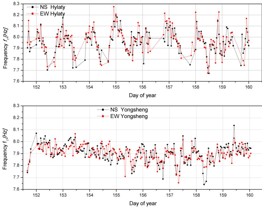
Fig. 2. Waveforms of hourly frequency values  $f_{1,NS}$  (black) and  $f_{1,EW}$  (red) of the first Schumann resonance mode determined on the basis of measurements conducted by the Hylaty ELF station (the upper graph) and Yon ELF station (the bottom graph) from 2011.05.31 (16:00 UTC) to 2011.06.09 (16:00 UTC).
