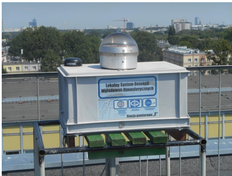
Fig. 2. The general view of LLDN-F(IGF) station located at the roof of IG PAS building. The GPS Garmin receiver and E-field antenna sensor mounted on the top of the grey box with the A/D recorder and the power supply buffer inside.
