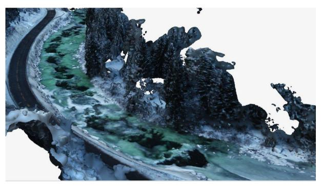
Fig. 1. Drone imagery of anchor ice damming a section of the river Sokna in Norway.
