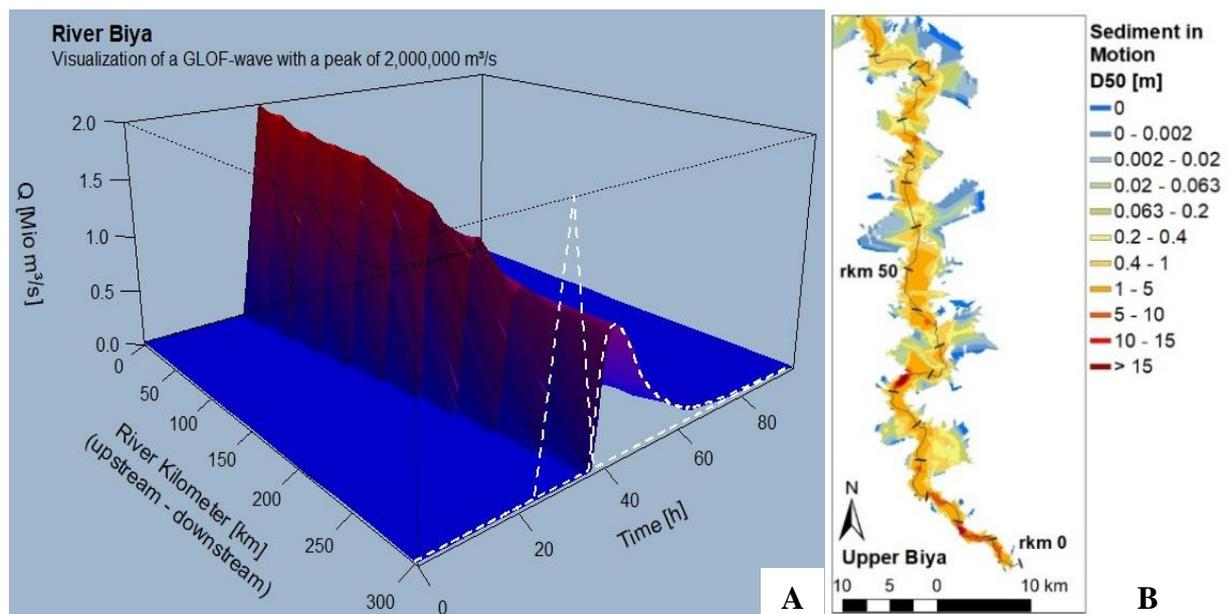
Fig. 1. Modeling results of the performed GLOF simulations.
