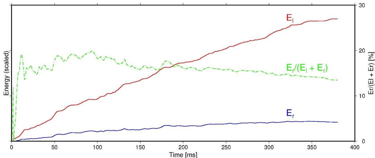
Fig. 3. Kinetic energies of linear ( $E_l$  – red line) and rotational ( $E_r$  – blue line) movements of particles. The ratio of rotational kinetic energy to the total kinetic energy ( $E_T = E_l + E_r$ ) is shown in green. Let us note that during the initial phase of the rupture development, this ratio reaches a considerable value of 20% which means that in this stage the rotational effects are quite important.
