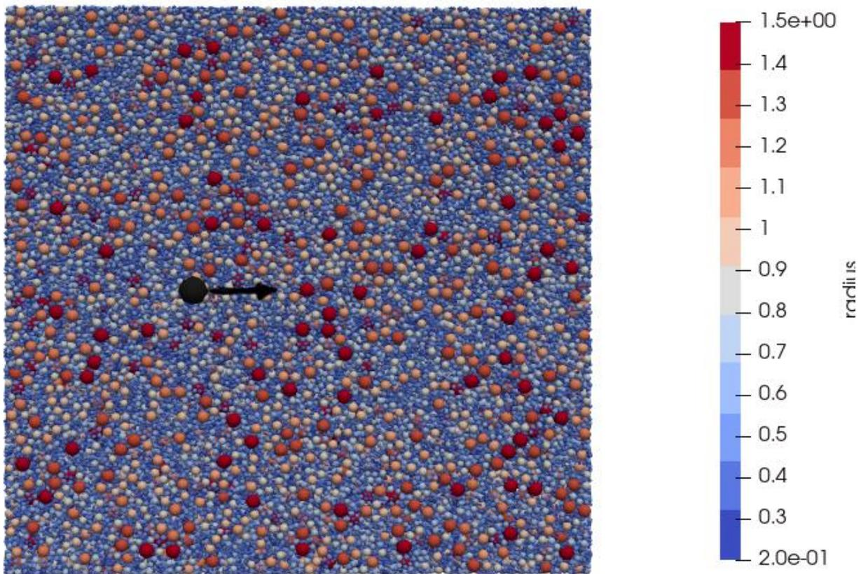
Fig. 1. Sketch of a numerical simulation setup designed for an analysis of rotational waves. The  $5\text{ cm} \times 5\text{ cm} \times 6\text{ mm}$  “rock” sample has been built of spherical particles with radii in the range  $0.2\text{--}1.2\text{ mm}$ . One of the particles (marked by black) starts to move right at the beginning of the simulation with a predefined velocity transferring energy to the plate.
