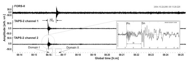
Fig. 2. Seismogram of the seismic events recorded on 22 October 2004 at 8 h 13 min by FORS-II and Second TAPS with two selected domains: Domain I where two channels of TAPS-2 detected classical seismic wave, and Domain II delayed about  $\Delta t_R$  where FORS-II detected rotational component. The insets show the method of time delay identification between *S*-waves (*Sn* line) and *P*-waves (*Pn* line) (from Jaroszewicz et al. 2006b).
