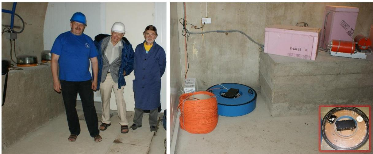
Fig. 3. July 2010: Prof. Jaroszewicz, Prof. Teisseyre, and an employee of the IG PAS Seismological Observatory in Książ (left photo) during the installation of the AFORS-1 in the measurement chamber at the Seismological Observatory in Książ (right photo) together with the view in the lower right window of the AFORS-1 destroyed by rats in July 2017.
