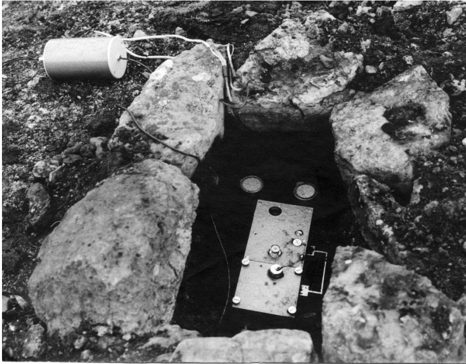
Fig. 2. Setting up the equipment and seismometer (1 s) of the IG PAS design, during research on Spitsbergen in 1976.
