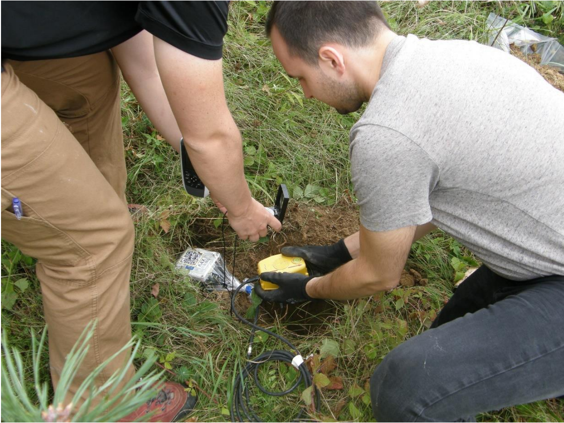
Fig. 22. Eng. Dariusz Wójcik, MSc, and his trainee set up a 3C (4.5 Hz) geophone with a CUBE recorder during measurements on the TTZ-South profile, 2018.
