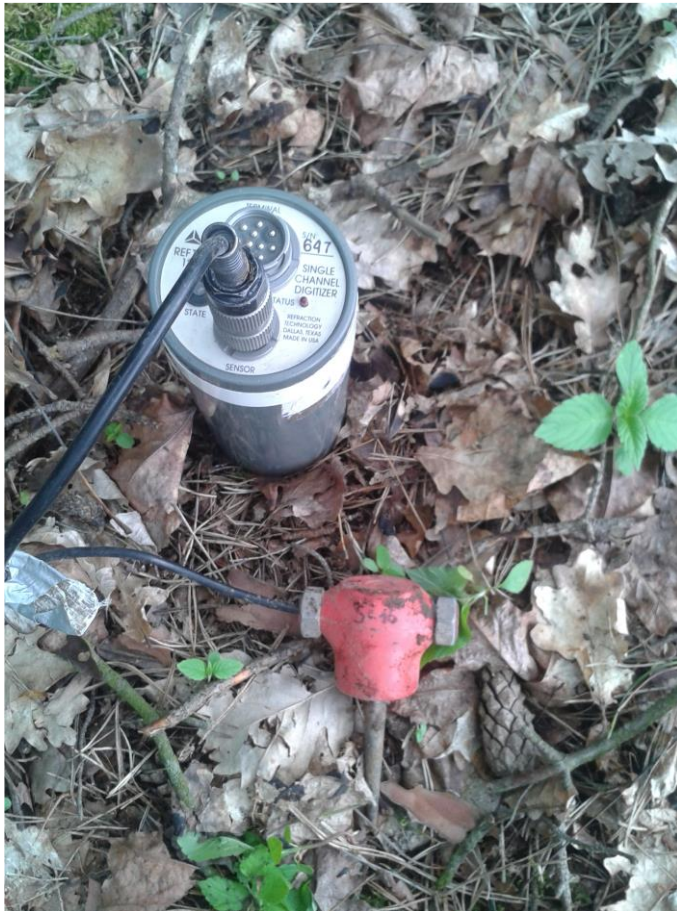
Fig. 18. Reftek 125 Texan (recorder) with geophone (4.5 Hz).
