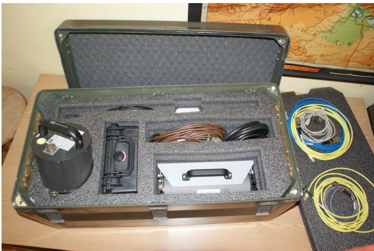
Fig. 29. Güralp CMG-40T broadband seismic apparatus (30 s), 2017.
