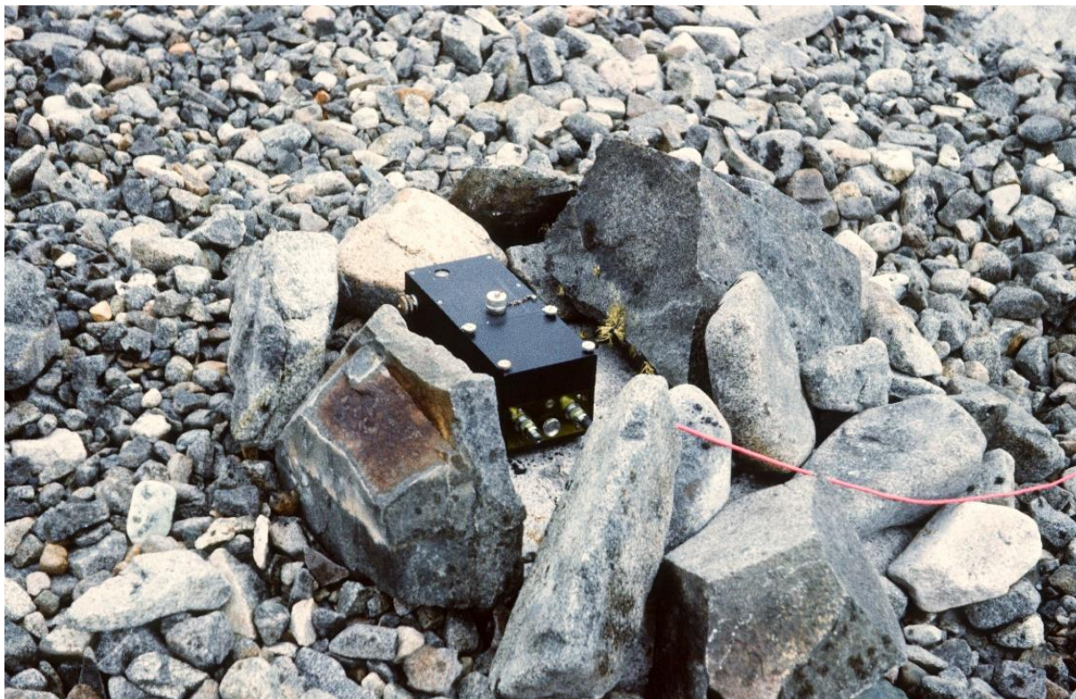
Fig. 4. Seismometer designed by IG PAS, manufactured by ZUD-GIG (SPI-70) (1 s), measurements in Antarctica.
