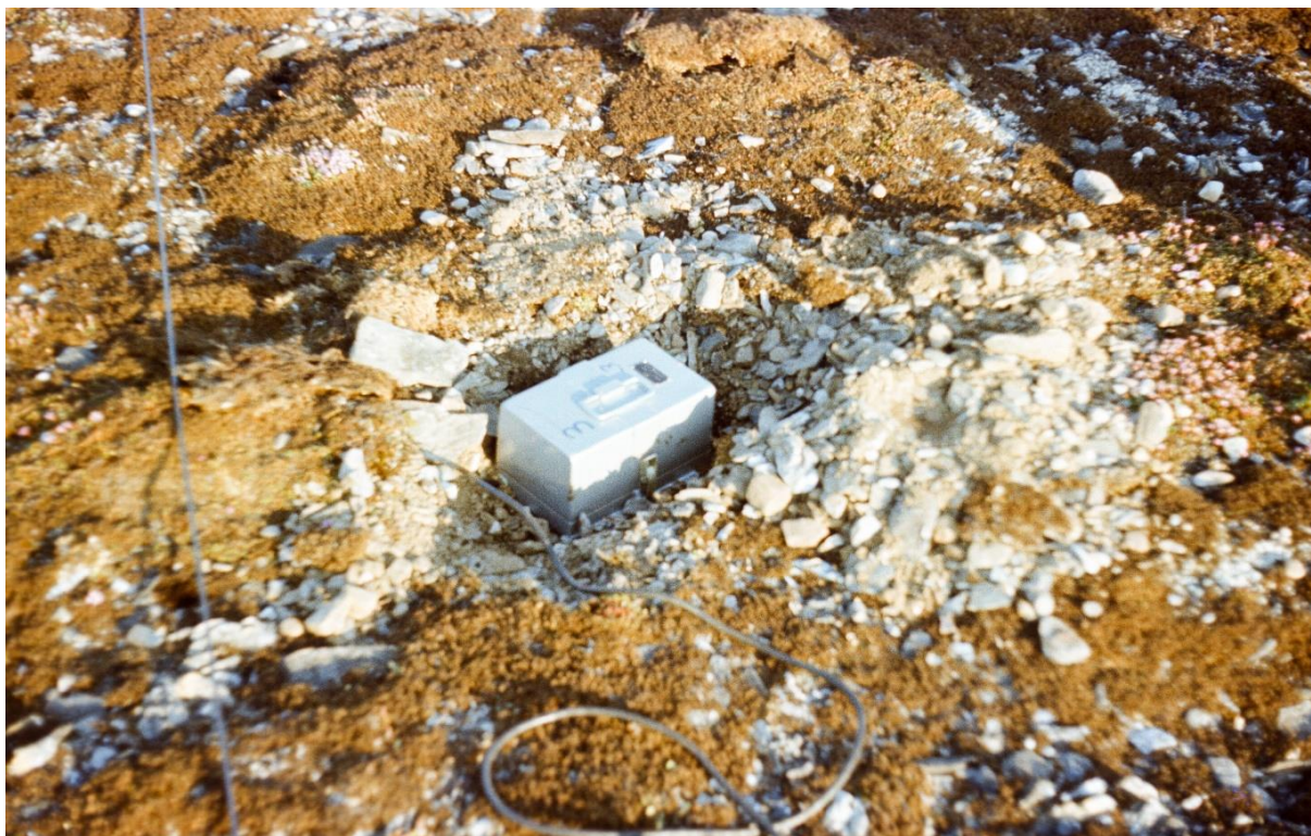
Fig. 6. SM-3, Soviet Union-made seismometer (1 s) during measurements on Spitsbergen, 1985.
