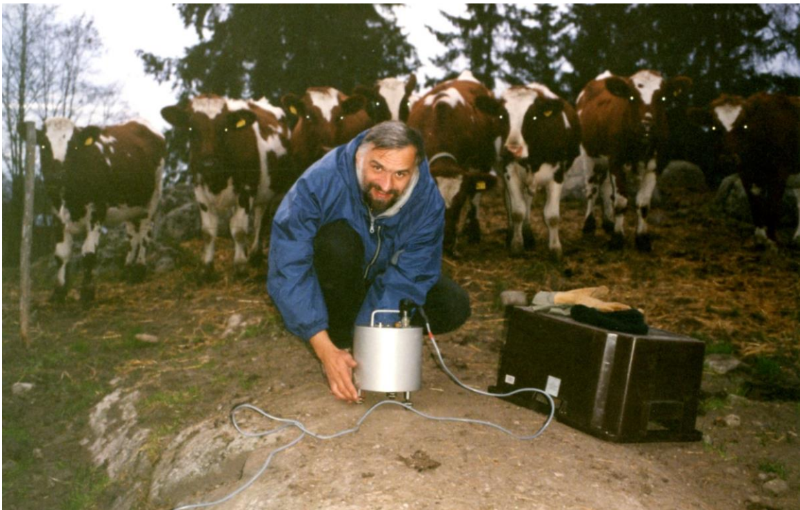
Fig. 13. Tomasz Janik setting up a Canadian-made 3C, Mark-L4C geophone, used alternatively with SM-3 seismometers for measurements with the MK-3 and MK-4P devices. Measurements during the SVEKALAPKO passive experiment, Finland, 1998.
