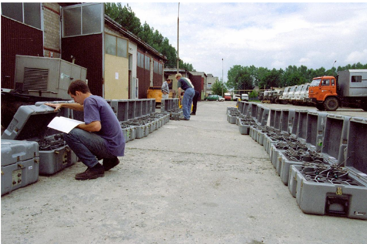
Fig. 15. Reftek 125 Texan short-period devices – preparations for measurements. The main base of the CELEBRATION 2000 project in Kraków.
