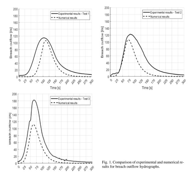
and real-world scenarios. The model incorporates critical flow conditions through the breach to calculate discharge, using formulations specific to triangular and trapezoidal cross-sections. The volumetric sediment load per unit width is determined using the Meyer-Peter Müller formula, assuming that critical shear stress is negligible compared to the mean shear stress.
