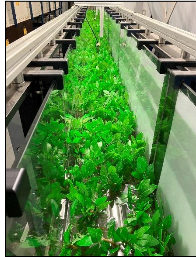
Fig. 2. Flume installation of realistic plants.
