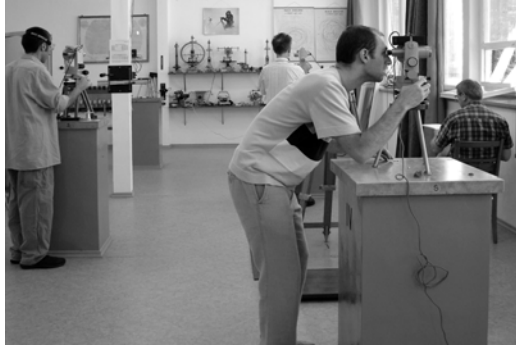
Fig. 3. Measurements with DI-flux magnetometers.
