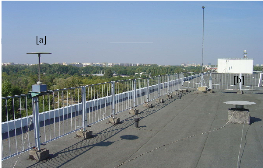
Fig. 1. The measuring site used for lightning event observations in Warsaw. [a] – the flat-plate antenna with frequency band 20 \text{ Hz} \div 1.3 \text{ MHz} and based on charge amplifier AD 711 having feedback time constant \tau = 5 \text{ ms} ; [b] – the Maxwell current flat antennae delivering the pulse of electric field change in the time domain, i.e. (\partial E/\partial t) , for the displacement current component of lightning flash events to be detected in the range of about 50 km from our measuring point and recorded by our data acquisition system. This system consists of 2-channel A/D PC 12-bit card having on its board a 64 MB memory buffer in each channel and triggered by the amplitude level of (\partial E/\partial t) signal, and the GPS time module unit giving the same time stamping 0.1 ms as the one used by the SAFIR/PERUN lightning detection network in Poland.
