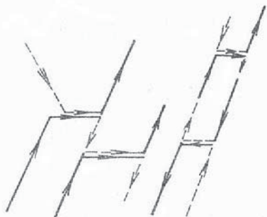
Fig. 3. A possible scheme of defect propagation in the dilatancy stage and in the convergency stage: same shear load
