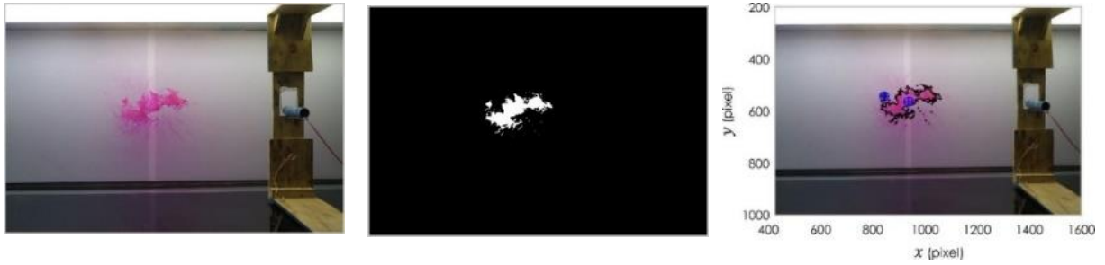
Fig. 1. Identifying the spill by imaging methods. From left to right: raw image, binary image, isolated spill.
