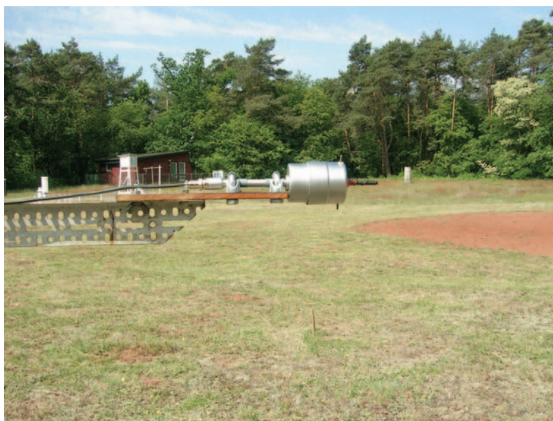
Fig. 3. Field-mill for the electric field strength measurement at Świder.
