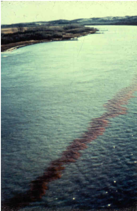
Figure 2.2: Tracer study of horizontal mixing in Missouri river in USA (river width: from B = 150 m to B = 240 m, maximum depth: H = 7.5 m); source: (Holley, 2001)
