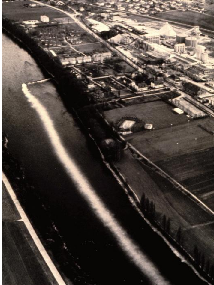
Figure 2.1: Aerial photograph (ca. 1960) of an industrial discharge located near the middle of the regulated River Rhine upstream of Lake Constance (Bodensee); photograph courtesy of D. Vischer, Zurich; source: ( Jirka & Weitbrecht, 2005 )
