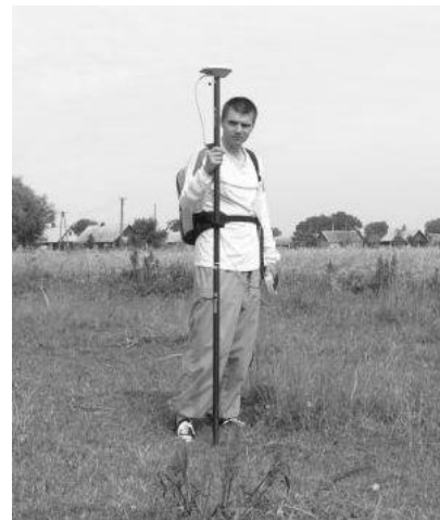
Fig. 3. The mobile set (rover).
