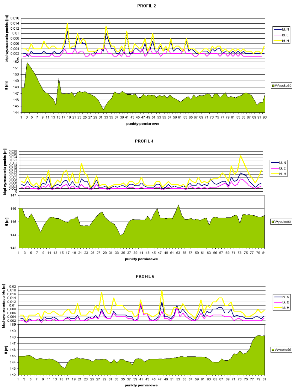
Fig. 8. Measured altitudes (ellipsoidal heights) on profiles 2, 4 and 6, and diagrams of errors of location components (NEH) determination in subsequent points.
