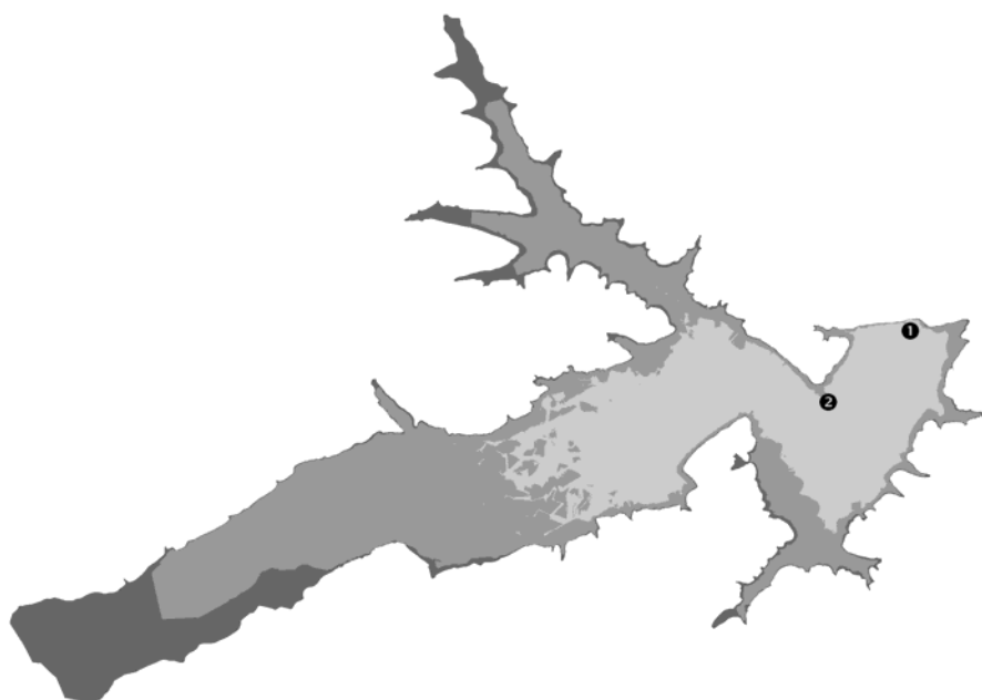
Fig. 1. The shape of the Dobczyce lake at different water levels: minimal (light grey), average (grey), and maximal (dark grey). The symbol ❶ shows the position of dam inlets while ❷ denotes the location of the water supply inlet.
