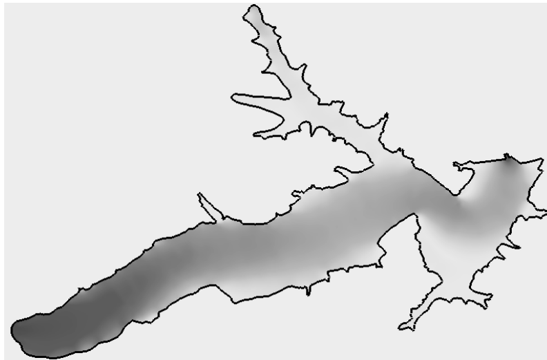
Fig. 3. Velocity map for 1560 \text{ m}^3/\text{s} flow at maximal water level. Arbitrary units, logarithmic scale on the z axis.
