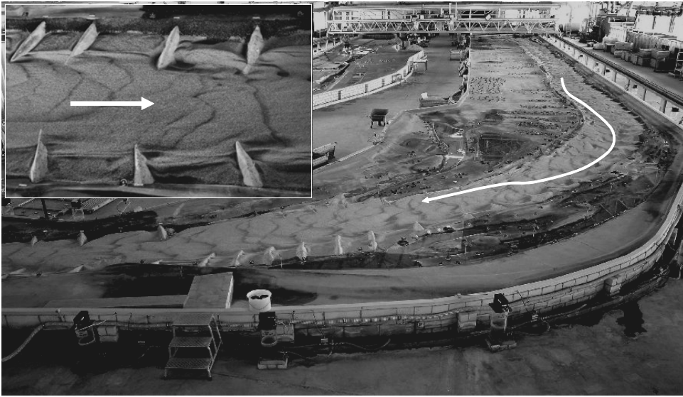
Fig. 1. Areal view of the bed-load-transport-model; detail of the river bed (inset). The arrows indicate flow direction.
