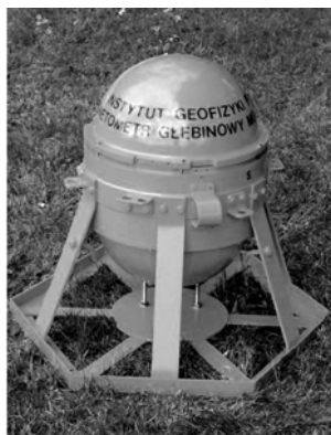
Fig. 1. The bottom magnetometer MG-01/2003 in its capsule.
