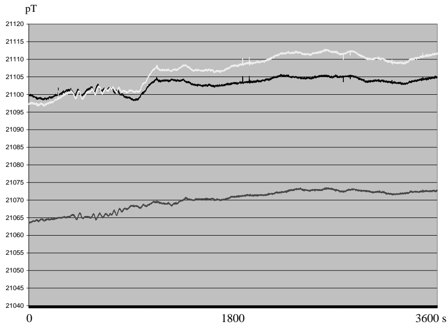
Fig. 7. Sample of SuperGrad total field record.
