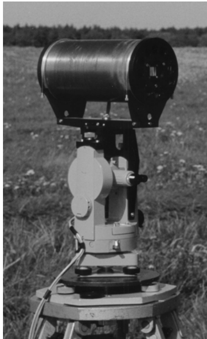
Fig. 1. Absolute measurement at repeat station with a PVM mounted on a non-magnetic theodolite.
