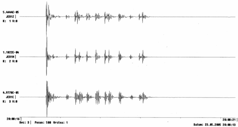
Fig. 7. Example of wave pattern of blast generated in the Jeroným adit.
