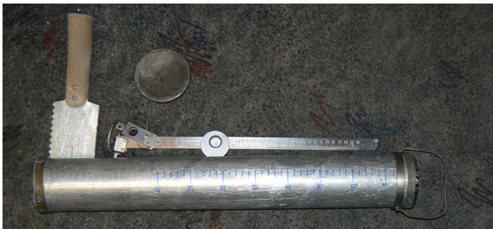
Fig. 29. Chomicz's snow tube sampler.
