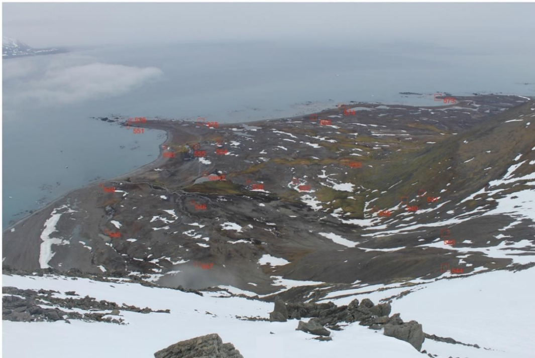
Fig. 34. Photo from the camera mounted on top of Fugleberget with marked location of all the GCP used in the orthorectification process.
