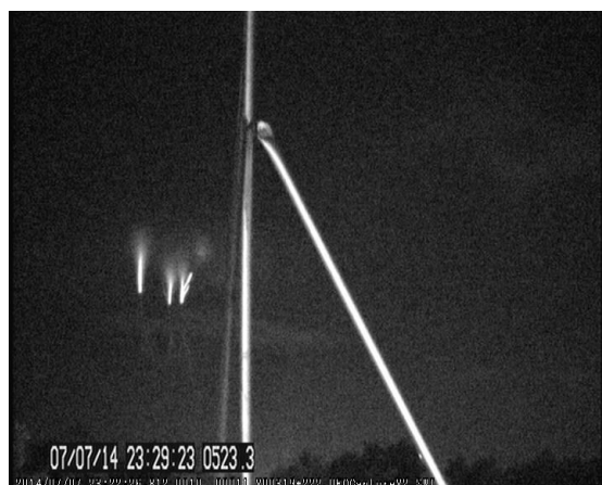
Fig. 1. Examples of TV frames consisting of two fields and their relevant on-screen display of PC time by UFOCapture (in the bottom line) and overlaid GPS timing by: a) KIWI-OSD at Gliwice and b) GPSBOXSPRITE-PIC-OSD at Świder. Note that the PC time label is illegible in the video fields due to interlacing.
