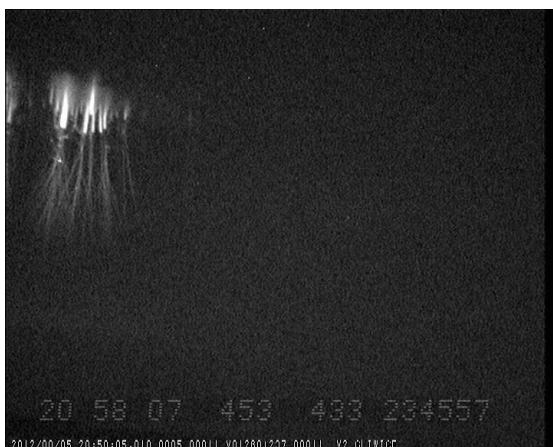
Fig. 1. Examples of TV frames consisting of two fields and their relevant on-screen display of PC time by UFOCapture (in the bottom line) and overlaid GPS timing by: a) KIWI-OSD at Gliwice and b) GPSBOXSPRITE-PIC-OSD at Świder. Note that the PC time label is illegible in the video fields due to interlacing.
