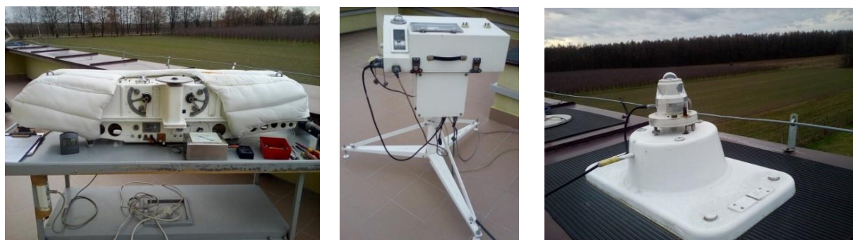
Fig. 1. Measuring equipment at the Belsk Observatory. From the left: Dobson spectrophotometer, Brewer spectrophotometer, UV-S-AE-T, Kipp & Zonen meter. Photos by P. Sobolewski.
