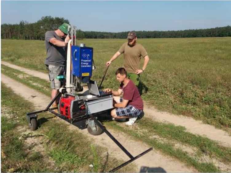
Fig. 1. Seismic source PEG-40 adapted to new carriage system, that can be operated without a car. This system can operate in rough terrain like steep hills and dense forest. Photo by M. Majdański.
