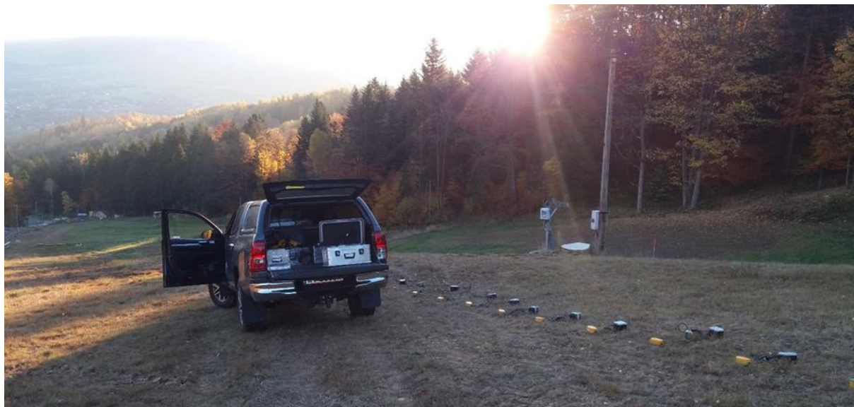
Fig. 1. The deploying of seismic line, with dense 1 m geophone spacing. The three component Omnirecs Stations allowed for gathering high-resolution geophysical data, which in near future deliver information about the evolution of the landslide in the Cisiec study site. The measurements conducted in October 2021, were part of long term research, aimed to investigate anthropogenic as well as climatic factors triggering the high mountain landslides development and evolution. The project is realized in cooperation with the Faculty of the Geology of the University of Warsaw and the Faculty of Natural Sciences of the University of Silesia as well as the Department of Magnetism of IG PAS (photo by Mariusz Majdański).
