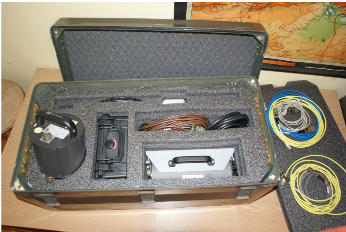
Fig. 29. Güralp CMG-40T broadband seismic apparatus (30 s), 2017.
