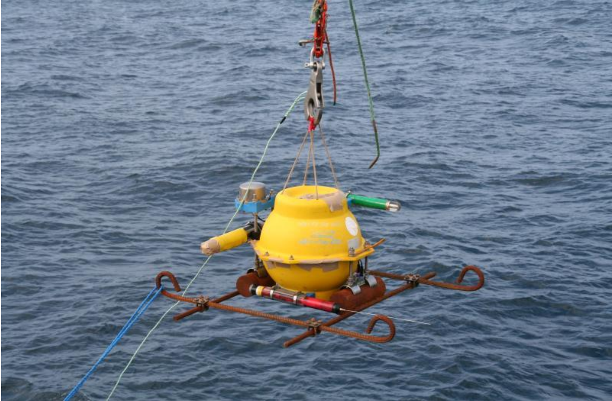
Fig. 24. Deploying of a Japanese OBS during the Horsted experiment, 2005 ( photo Wojciech Czuba ).
