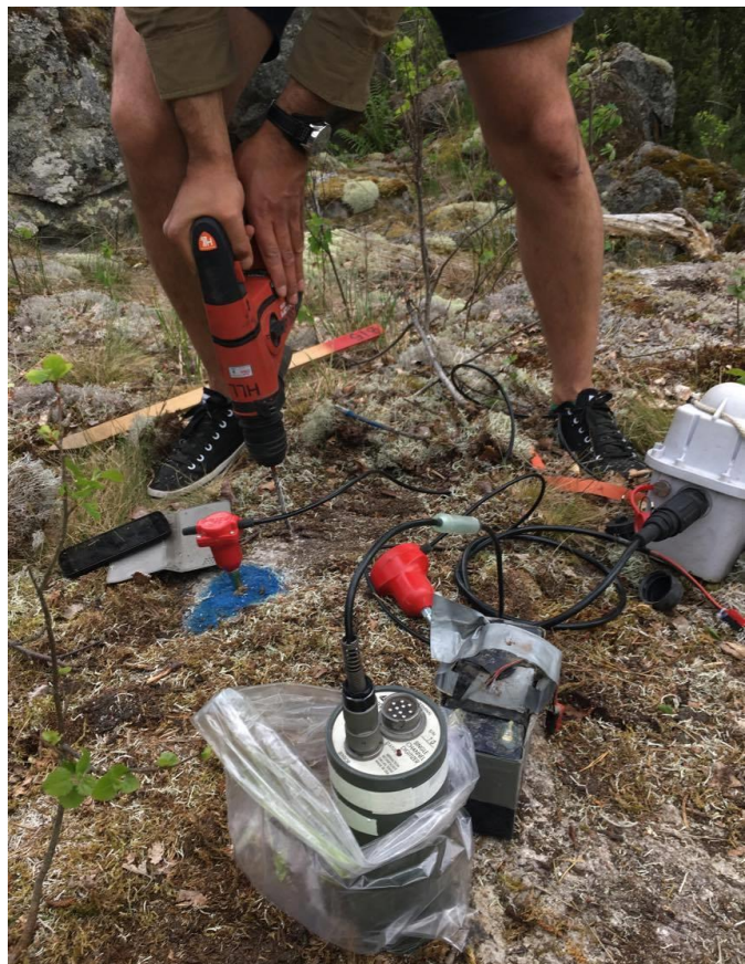
Fig. 19. Drilling holes in the rock bed for the geophone pins of the Reftek 125 Texan. Profile UPPLAND (BASIC), southern Sweden, 2017 (photo Dariusz Wójcik).
