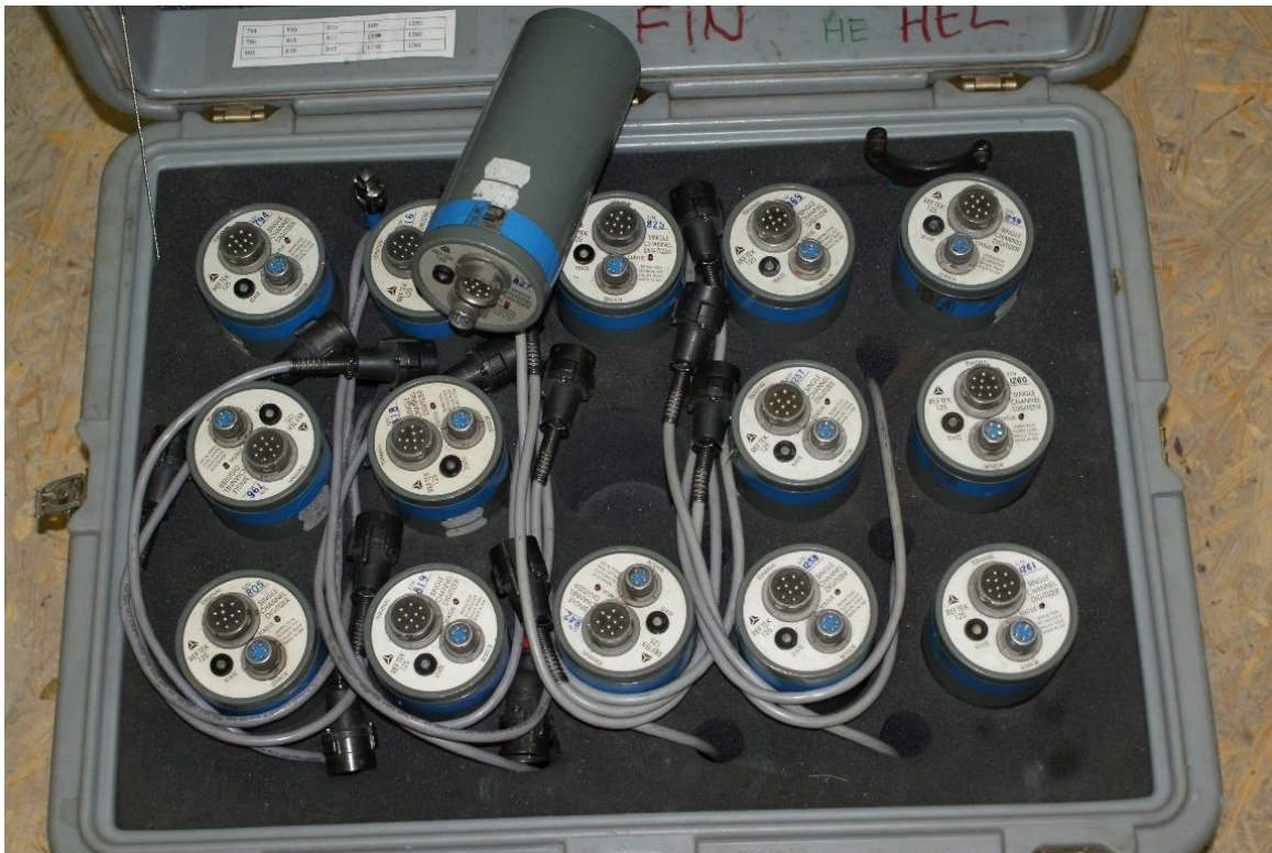
Fig. 17. Transcase with 15 Reftek 125 Texan field seismic short-period devices. Used by our team since 1997 until now. Initially only rented, and since 2000 also owned.
