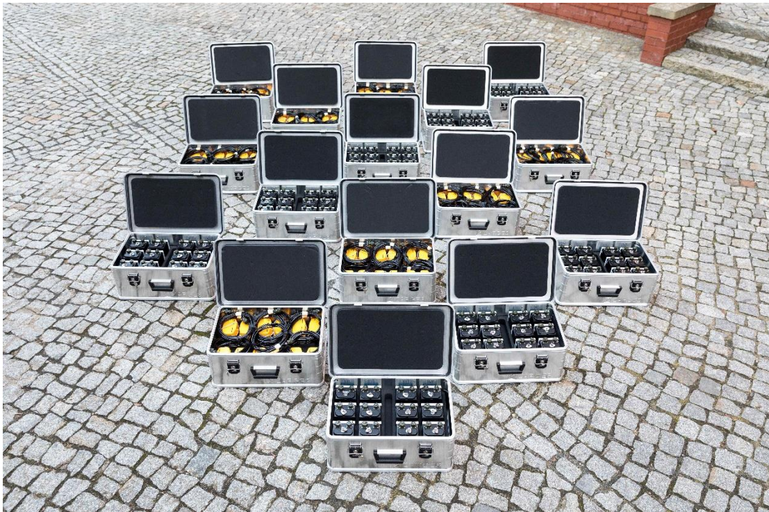
Fig. 21. A set of 100 short-period CUBE 3C field seismic stations with three-component geophones. Used since 2013.
