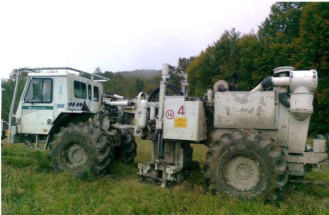
Fig. 31. One of the Geofizyka Toruń vibrators working on a deep reflective profile POLCRUST-01, 2010.
