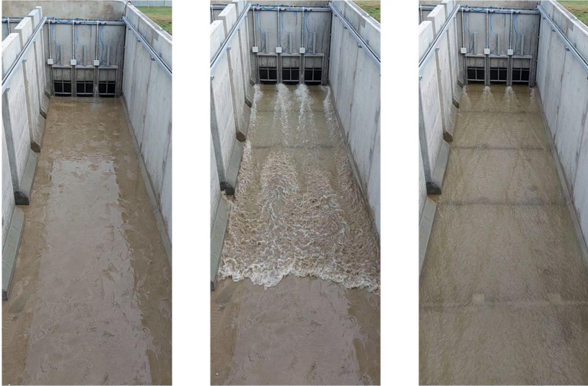
Fig. 2. Effectiveness of substrate leaching on the real model at the preset filling T = 2.4 m in the reservoir damming chamber and the assumed opening of the sluice gates a = 0.2 m. Sediment flushed out at 100%. View of one track without applied walls.
