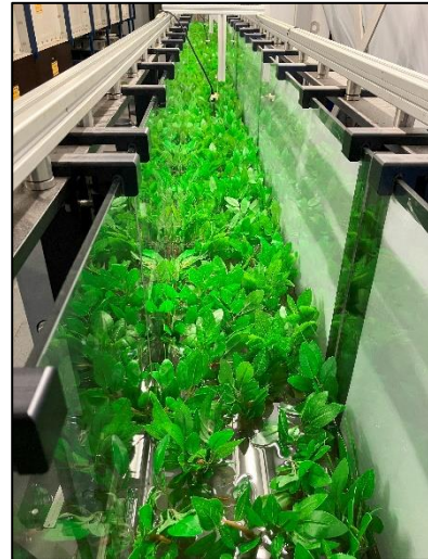
Fig. 2. Flume installation of realistic plants.
