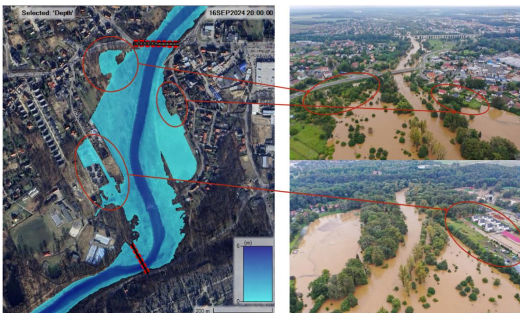
Fig. 3. Comparison of the results for the September 2024 flood, performed using the Full Model DWE, with the actual flood situation shown in the photos presented in Miasto Bolesławiec (2024).
