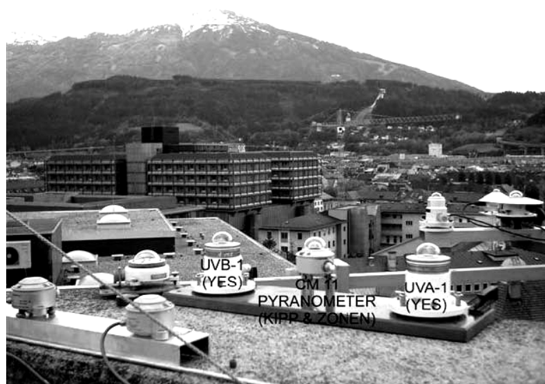
Fig. 2. Comparison of the IGF PAS traveling UV calibration system with the Bentham spectrophotometer DM 150 in Innsbruck in May 2006.
